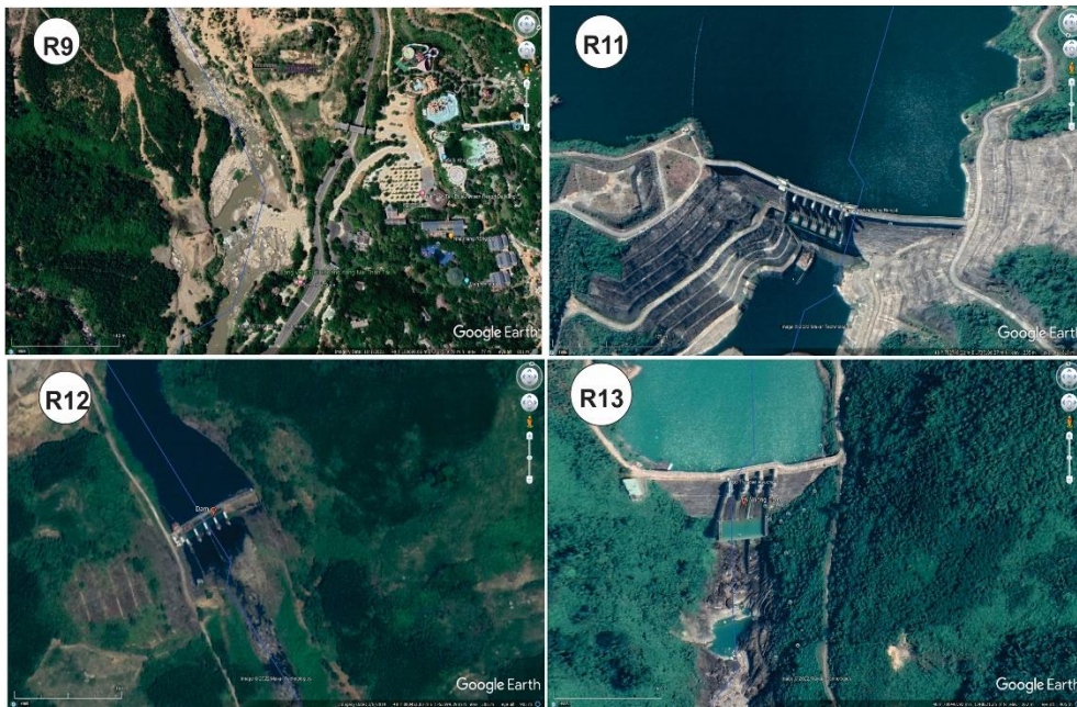
Figure 4. Examples of artificial (dam-induced) knickpoints on the R9, R11, R12 and R13 river profiles, confirmed on Google Earth imagery.
